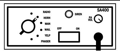
The **OFF/ON** Rocker Power Switch controls the siren power. The siren may be left on any time the vehicle is in operation. The power should be turned off when vehicle is not being used to conserve battery power.
